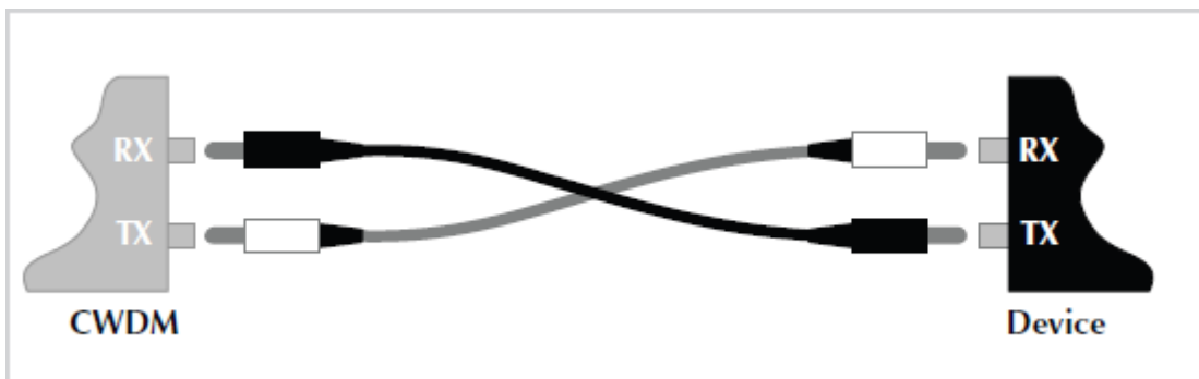
Figure 7: Fiber Cable Connections
