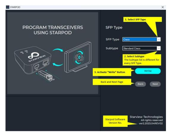
After selecting the "SFP Type", choose the correct subtype (if any) before clicking the "Write" button to start the recoding process.
