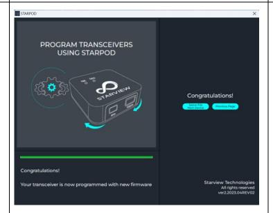
When you receive this congratulatory message, the programming of the coding into the transceiver EEPROM is considered successful and you can start using the transceiver module in your equipment.
