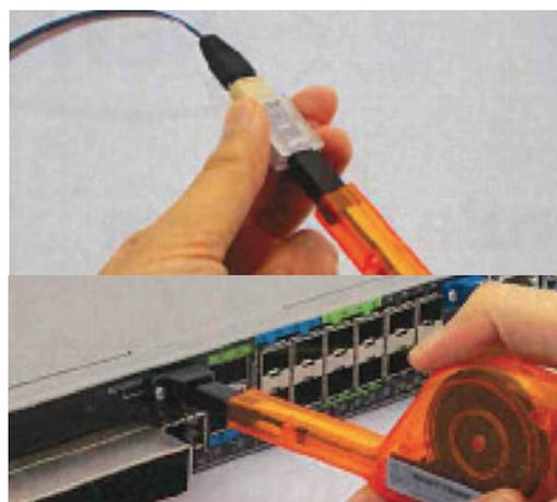
The Smart Cleaners are dry cloth cleaners specially designed to clean single fiber connectors residing in an adapter, faceplate or bulkhead. The Smart Cleaners are simple to use and highly effective at removing oil and dust contaminants that can negatively impact optical performance.
