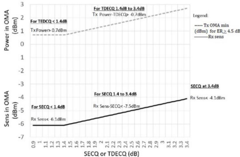
Figure 4. Illustration of Receiver Sensitivity Mask for 4x100G LR
